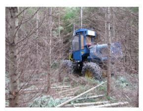
Rottne 2002 "mini-harvester". This machine is less than 8 feet wide and can reach about 23 feet with the harvester head. The machine is shown operating in an overgrown grand-fir Christmas tree plantation in Bonners Ferry, Idaho on private lands in 2008. Photo by Barry Wynsma, USFS October 2008
