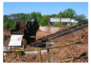
The Scotts Company, Naturescapes mulching operation, Waverly, Virginia. Trucks are dumped by hydraulic lift or vans that use moving floors, then material is sorted into piles and conveyors for processing. May 18, 2006. John Stewart
