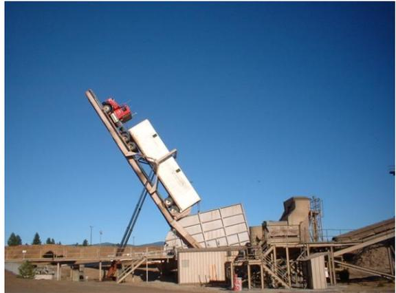
*Chip truck off-loading via hydraulic lift at the Mt. Lassen Power plant, Westwood, California. September 18, 2002.
