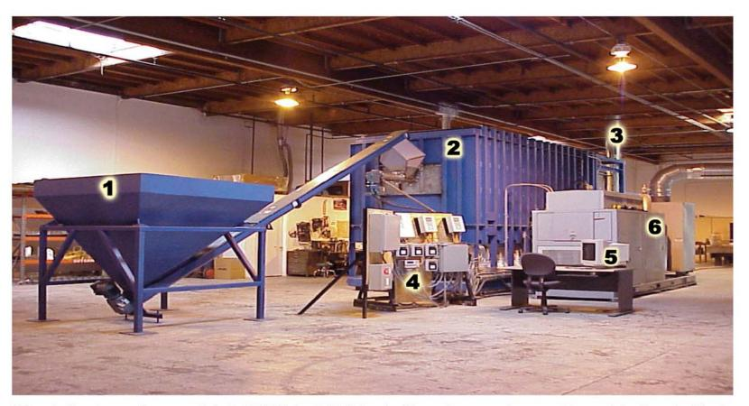
This photo shows the completed 250kW test Unit in AgriPower's current assembly and testing facility in Sacramento, California. The automated feeder hopper module (1) on the left is connected to the combustion chamber module (2). The heat exchanger module (3) is in the right rear. The control panel (4) is in the center, the operating computer (5) is in the immediate front and the turbine generator set (6) is behind the computer.
