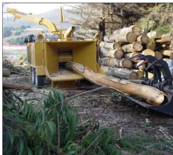
Large sections of eucalyptus are mechanically loaded into the new, heavy duty chipper during a fuel reduction project at Fort Barry.
