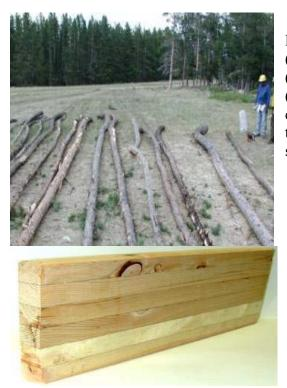
This 1.5- by 9-inch Lam Lumber beam will form the web section of an I-Beam. Laminated flanges will be formed and bonded to the top and bottom of the web. Curved lumber will thus be laminated into a straight beam.
