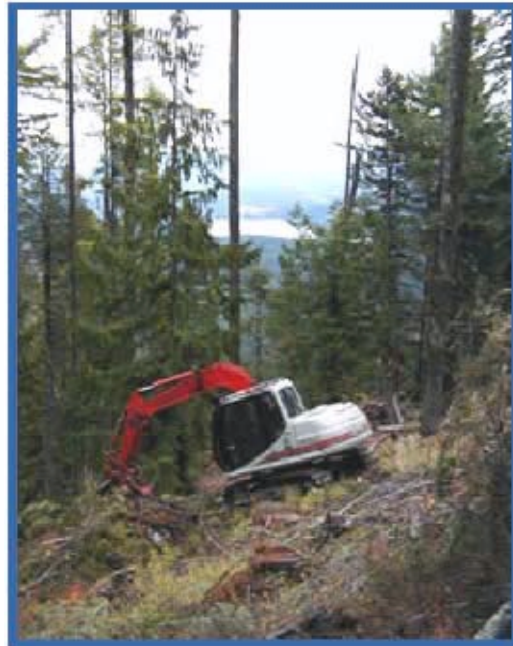
Machine piling logging slash and hazardous fuels.
