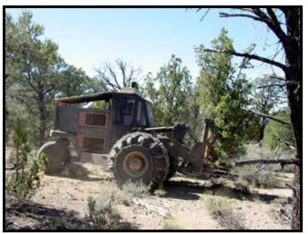
BLM-contracted crews utilized two three-wheeled Feller Bunchers to selectively thin and stack the pinyon-juniper. The accumulated woody vegetation was later chipped, resulting in nearly 9,000 tons of biomass. Slated for eventual sale, the biomass is currently being made available to the public for use in landscaping and other efforts.
