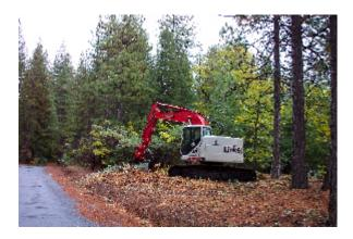
Brush mastication was accomplished along primary transportation routes with the machine displayed here. Standing brush and small trees are mulched down to a low compact fuel bed.
