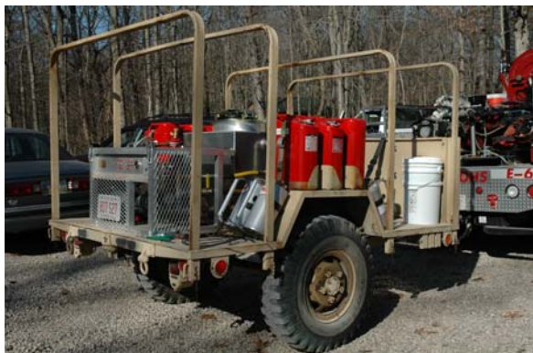
Ohio DNR uses a trailer acquired through the Federal Excess Personal Property Program to carry burning equipment. The drip torches, terra-torch, and fuel container were purchased with NFP funding. Photo courtesy Ohio DNR
